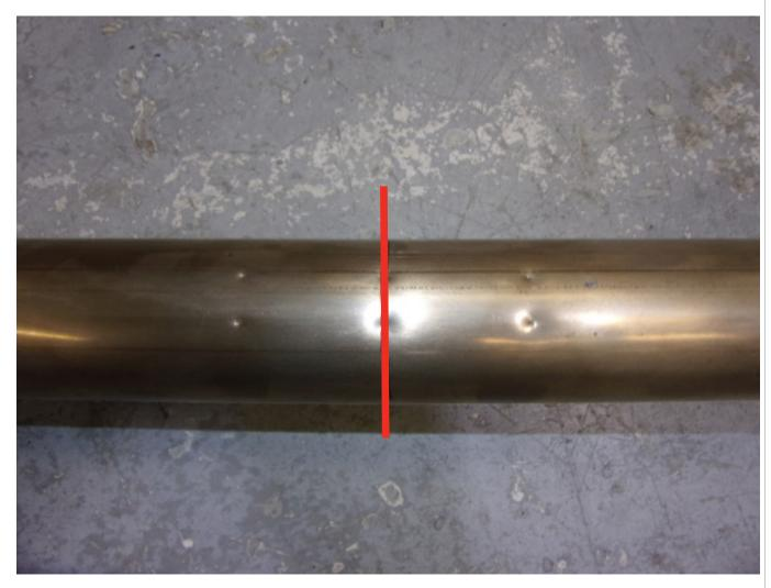
To make it easier to cut the exhaust we reccomend removing it from the car. Find the 3 pairs of indents and use the middle pair to mark out the cutting line. Cut along the line and de-bur the edges. Re-fit the original GPF and fit the Scorpion GPF-back following the line diagram above. NOTE: If fitting at the same time as our GPF delete you won't need to cut the system.
